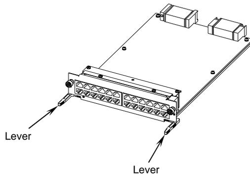
2. Hold the levers and slide the optional unit slowly into the device until the levers touch the device.
