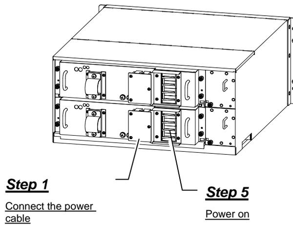
AX6608S (using the AC power supply)
