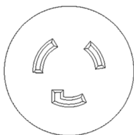
Figure 2-7 Two-pin grounded twist-lock outlet (250 V, 20 A)
