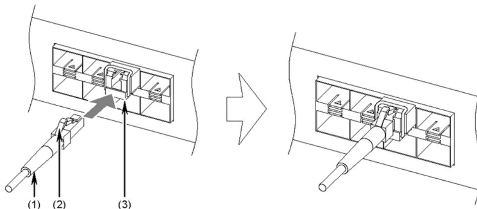
(1) Fiber optic cable (LC simplex connector)
