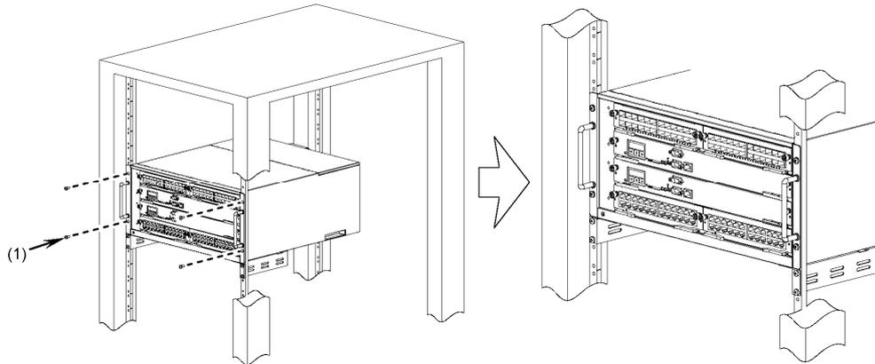
(1) Screws (M5 or M6 x 4) supplied with the rack
