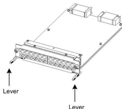
2. While holding the levers, push the optional module carefully until the levers touch the Switch.
