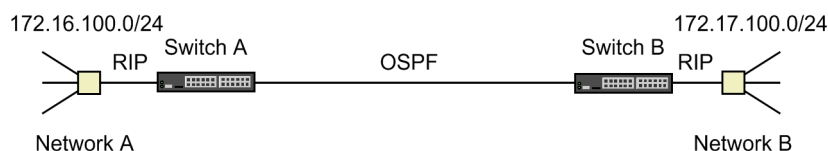
Figure 7-3: Connections between subnets with different network addresses
