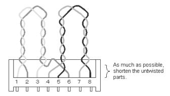
Note that the 1000BASE-T loop connector above is only supported for loop operation for the Switch. (Loop operation by the 1000BASE-T connector is a non-standard, proprietary action.)
