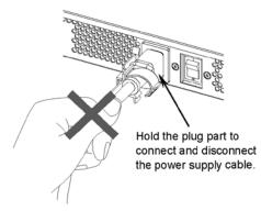
• When connecting or disconnecting a DC power cable, always hold the connector of the cable. Pulling the cable itself might cause the wires to break.
