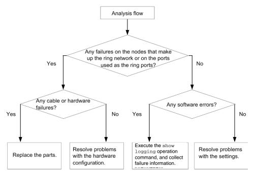
If operation cannot be performed correctly or a ring network failure is detected when the Ring Protocol is used, use the failure analysis method described in the table below to isolate the cause of the problem for the relevant node in the target ring network.
