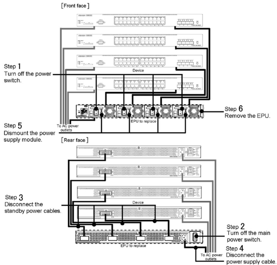
**Figure 4-56** Replacing an external redundant power unit (EPU-D)
