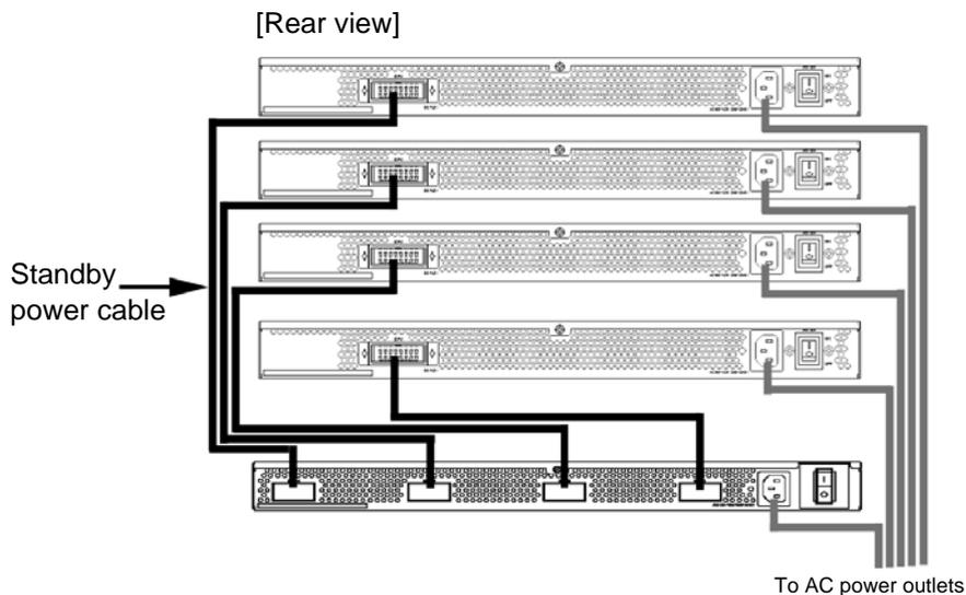
**Figure 4-25** Connection schematic of the standby power cable (Connecting the external redundant power unit EPU-D to the DC model)
