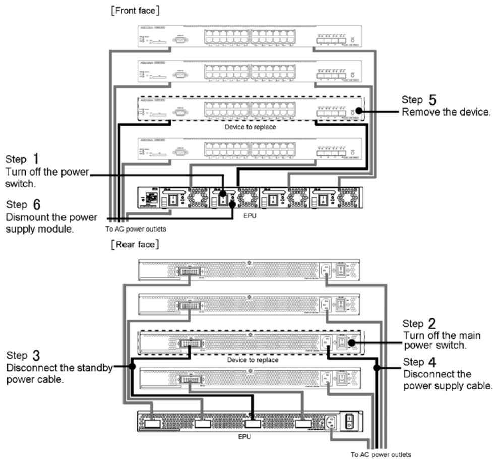
**Figure 4-54** Removing the Switch (DC model)
