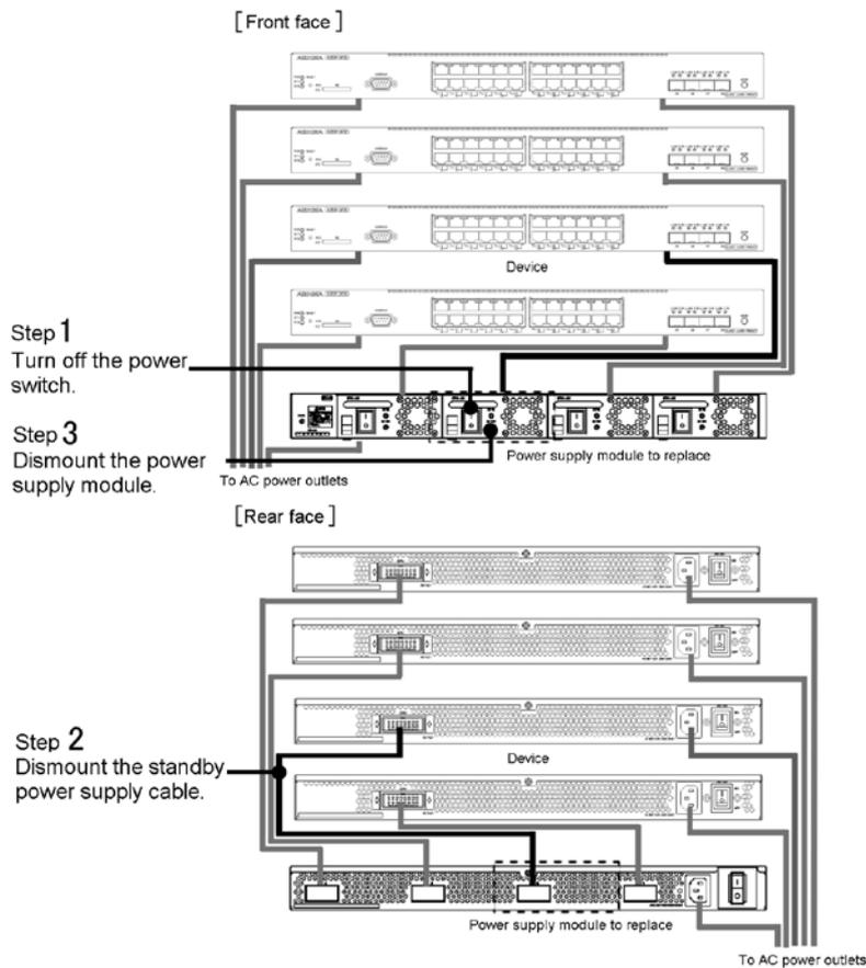
**Figure 4-58** Replacing power supply modules (EPU-DM)
