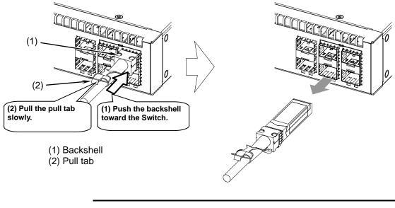
Figure 4-14 Disconnecting a direct attach cable
