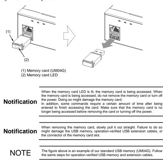
Figure 4-9 Removing UM04G
