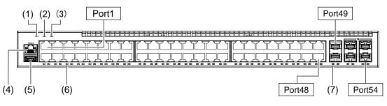
**NOTE** Direct attach cables can be used only for Port 53 and Port 54.
