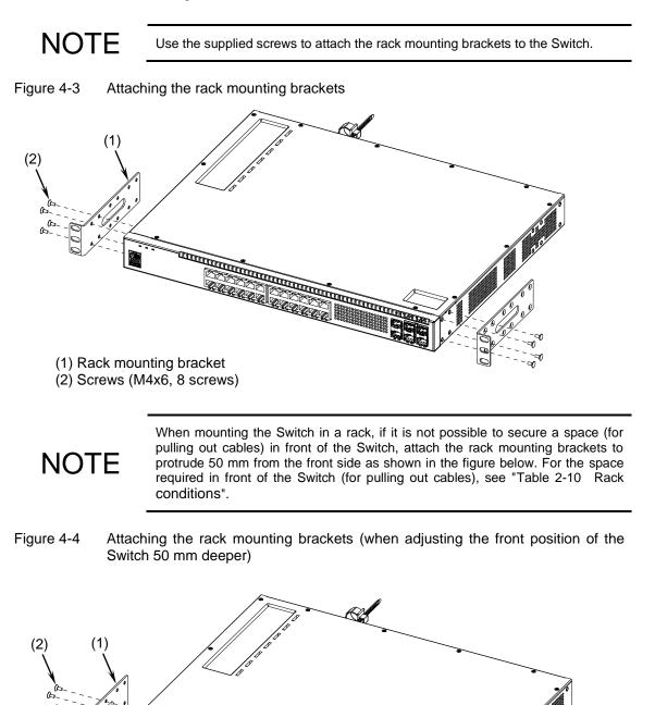
(1) Rack mounting bracket (2) Screws (M4x6, 8 screws)
