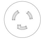
If you do not use the 200 V AC power cable that we sell separately, use the outlet below. The outlet is available at most electrical installation stores.
