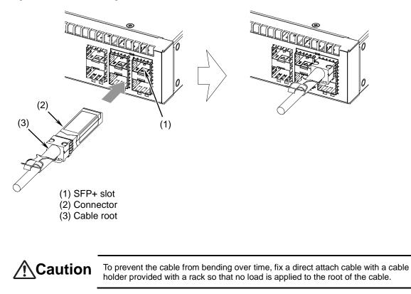
The figure above is an example of connecting the cable to an upper SFP+ slot. When connecting the cable to a lower slot, insert the connector upside down.
