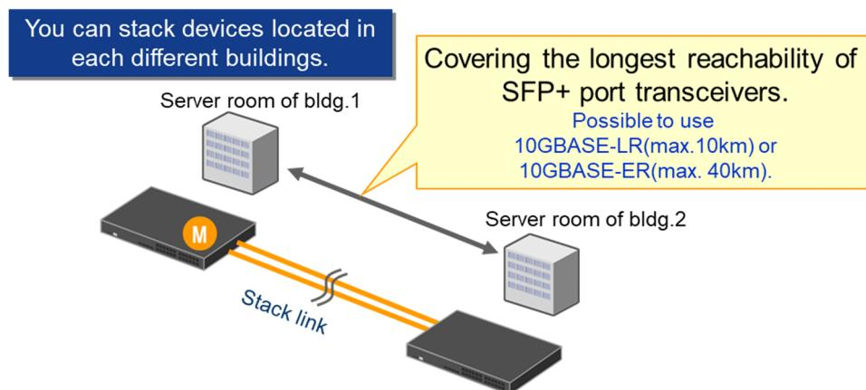
**(4) Establish a stack link by directly connecting the member switches to each other.**
