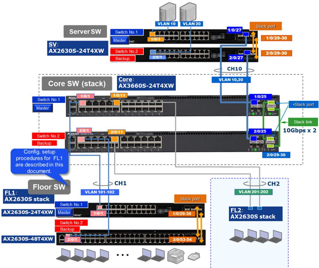
The configuration/setting tips in L2 stack here are the same as the tips described in [3.1.2 Configuration tips](#) and [3.1.3 Setup tips](#), except for the floor switches. Note the following configuration tips when applying L2 stack to the floor switches.
