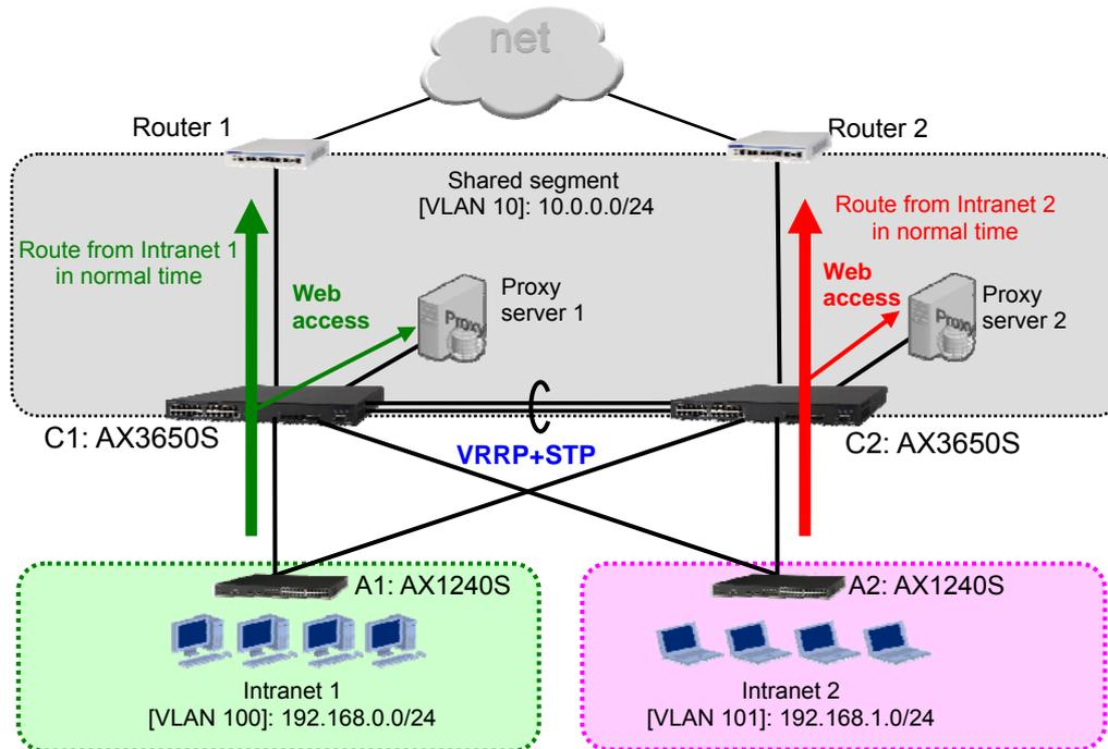
**Figure 3.1-1: Example of a redundant system using proxy servers**
