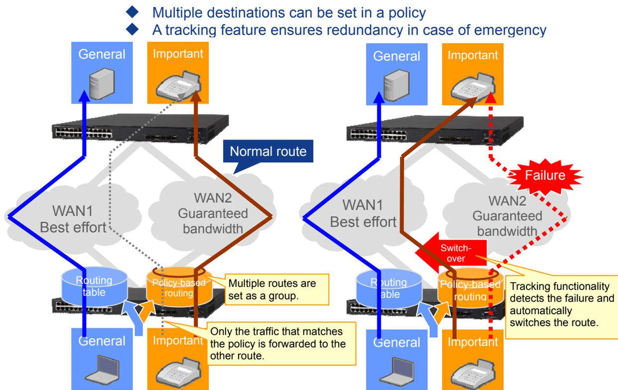
**Figure 1.2-1: What can be done with the policy-based routing in the AX series**
