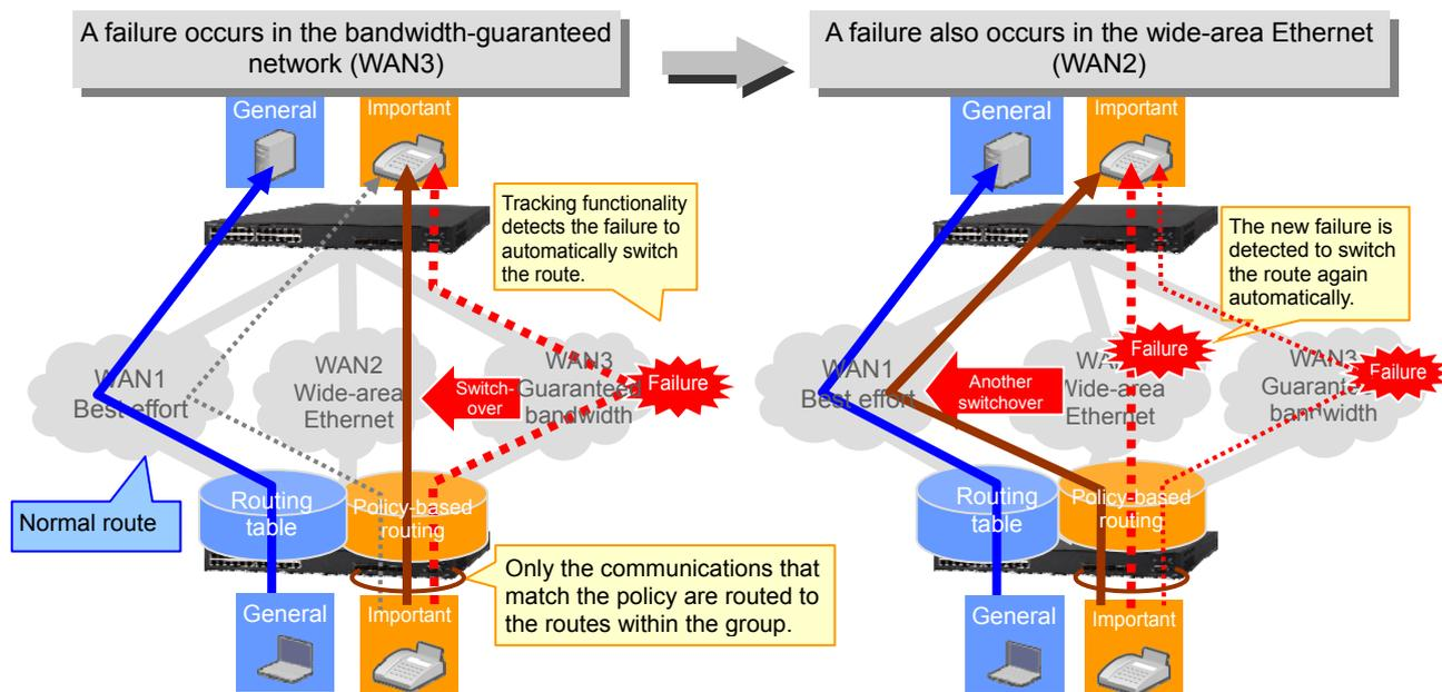
Figure 2.2-1: Example of forwarding only IP telephone traffic
