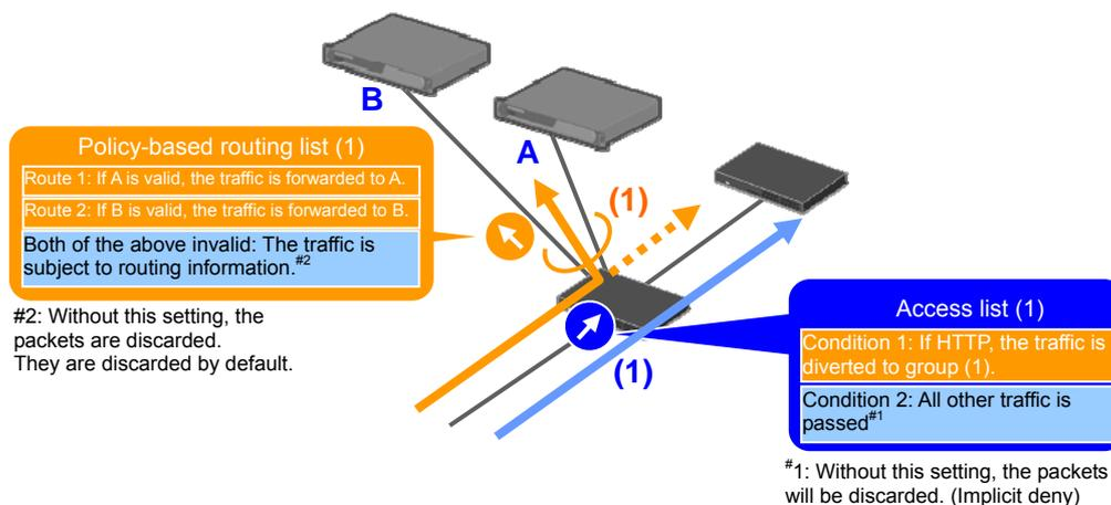
**Figure 3.1-3: Default behaviors of the access list and the policy-based routing list**
