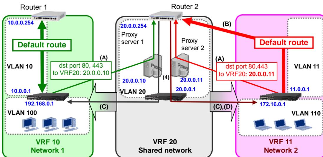
Figure 3.2-4: Image of the example policy-based routing configuration
