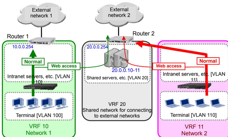
**Figure 3.2-2: Configuration image of the logical network**
