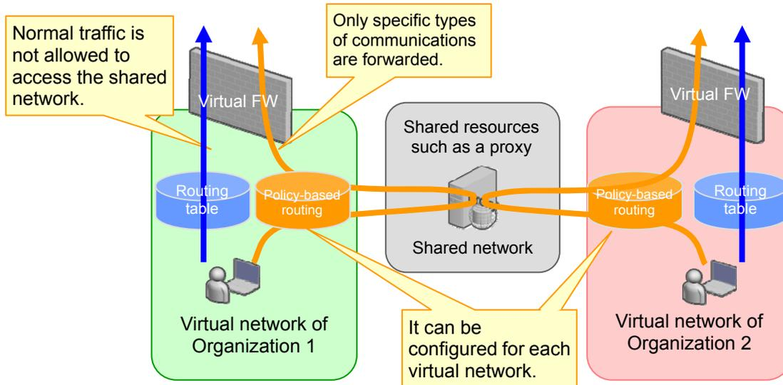
**Figure 1.2-2: Securing shared networks with policy-based routing**
