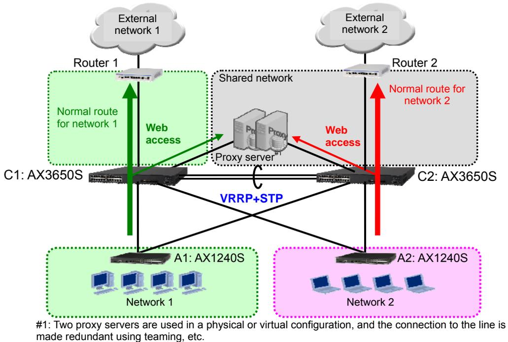
**Figure 3.2-1: System example in which network partitions are used (physical configuration)**
