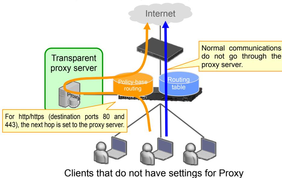
**Figure 2.1-1: Example of forwarding only Web access to the proxy server**
