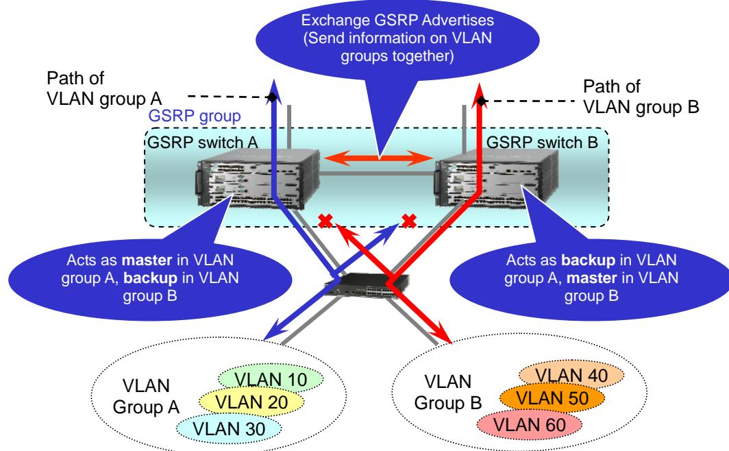
Figure 2.1-2 GSRP's load balancing
