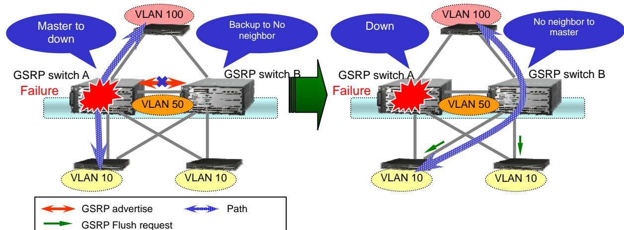
Figure 1.2-2 Operations at the time of master device failure
