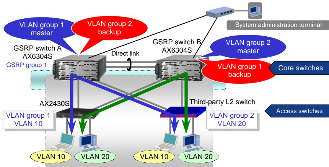
Figure 2.1-1 Load-distributed GSRP configuration
