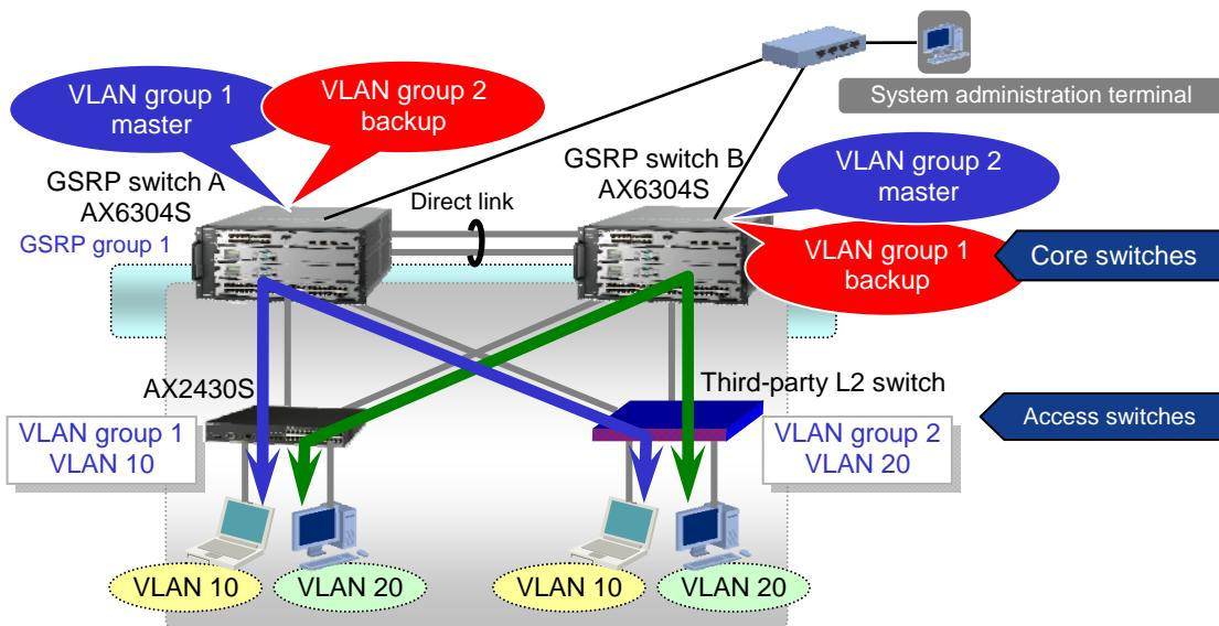
**Figure 2.1-1 Load-distributed GSRP configuration**
