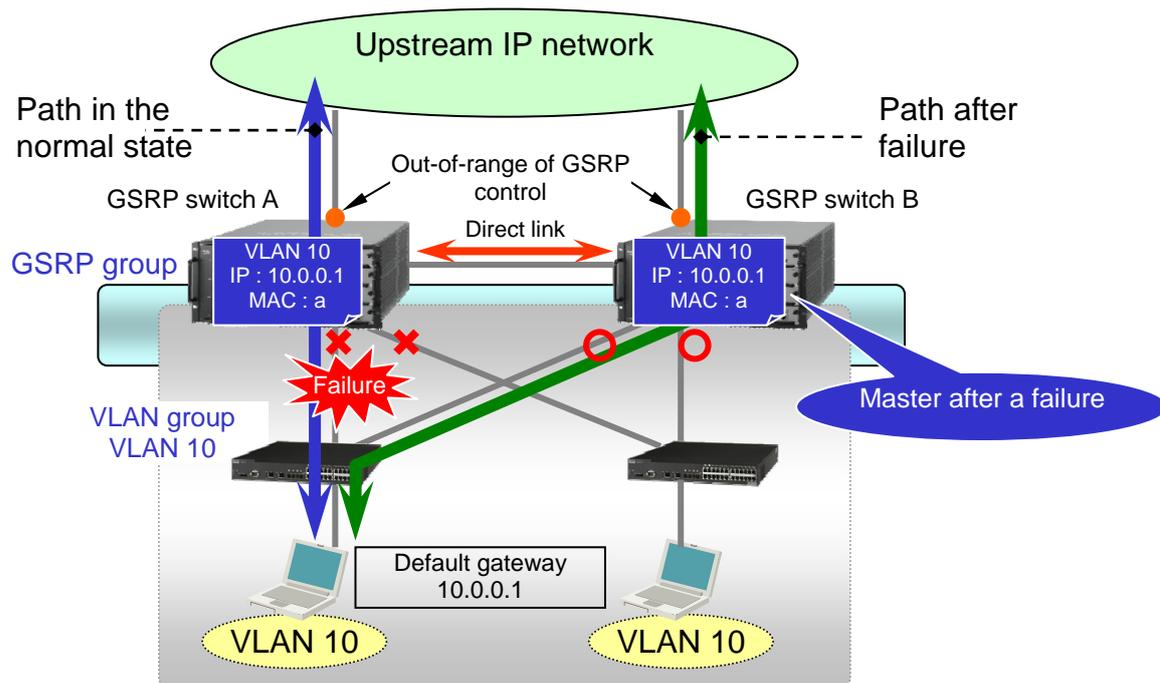
Figure 1.1-1 Layer 3 redundancy switching
