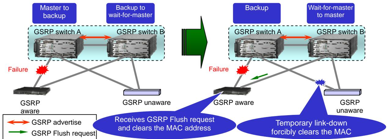
Figure 1.2-1 Operations at the time of link failure
