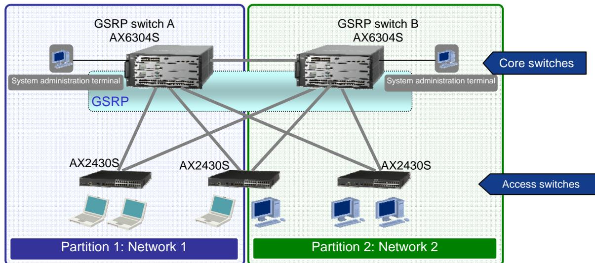
Figure 3.1-1 A network separation system utilizing Network Partition
