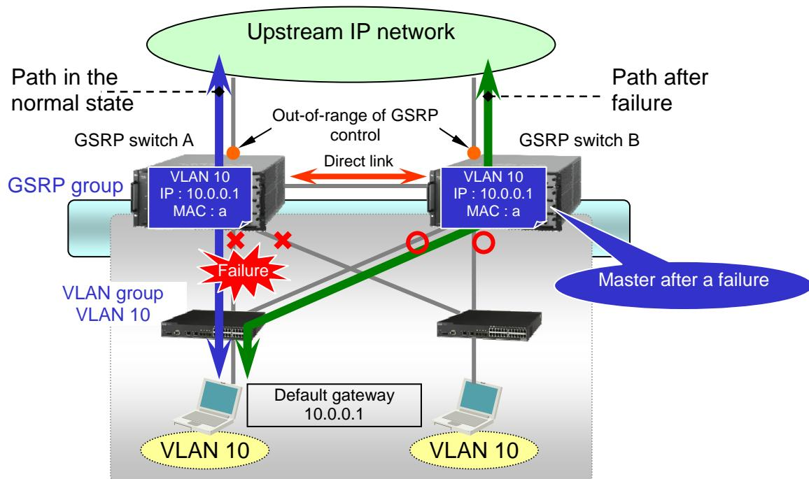
**Figure 1.1-1 Layer 3 redundancy switching**
