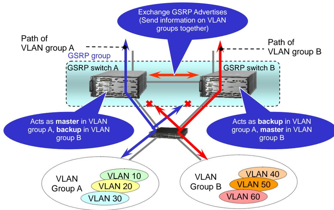
Figure 2.1-2 GSRP's load balancing
