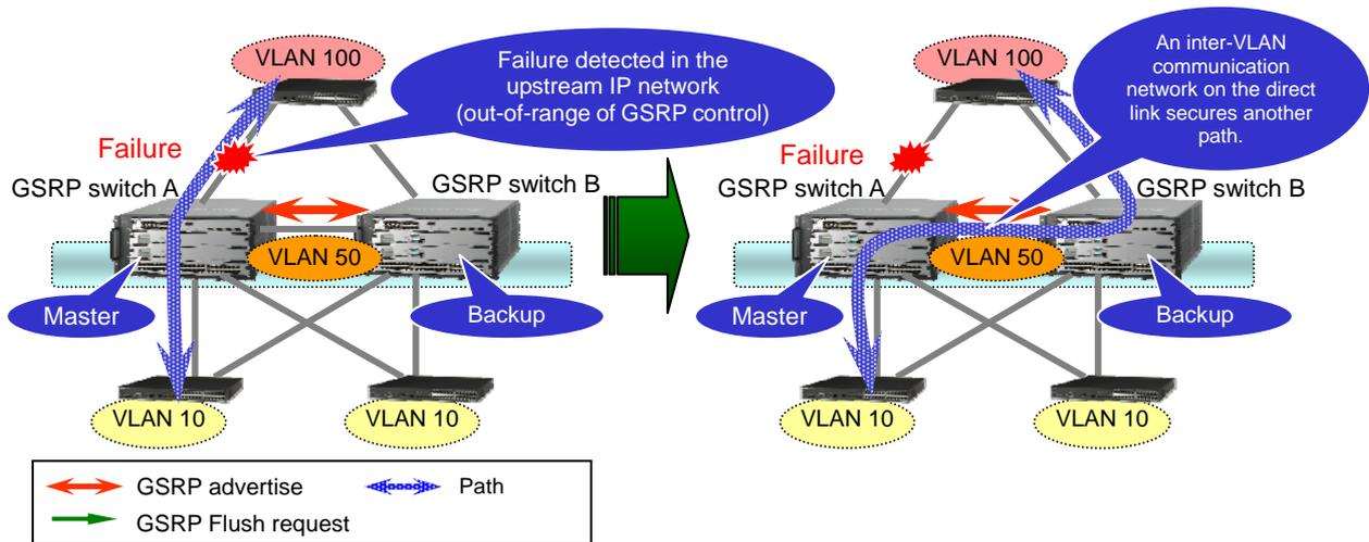
**Figure 1.2-3 Operations in case of a line failure with an upstream IP network**
