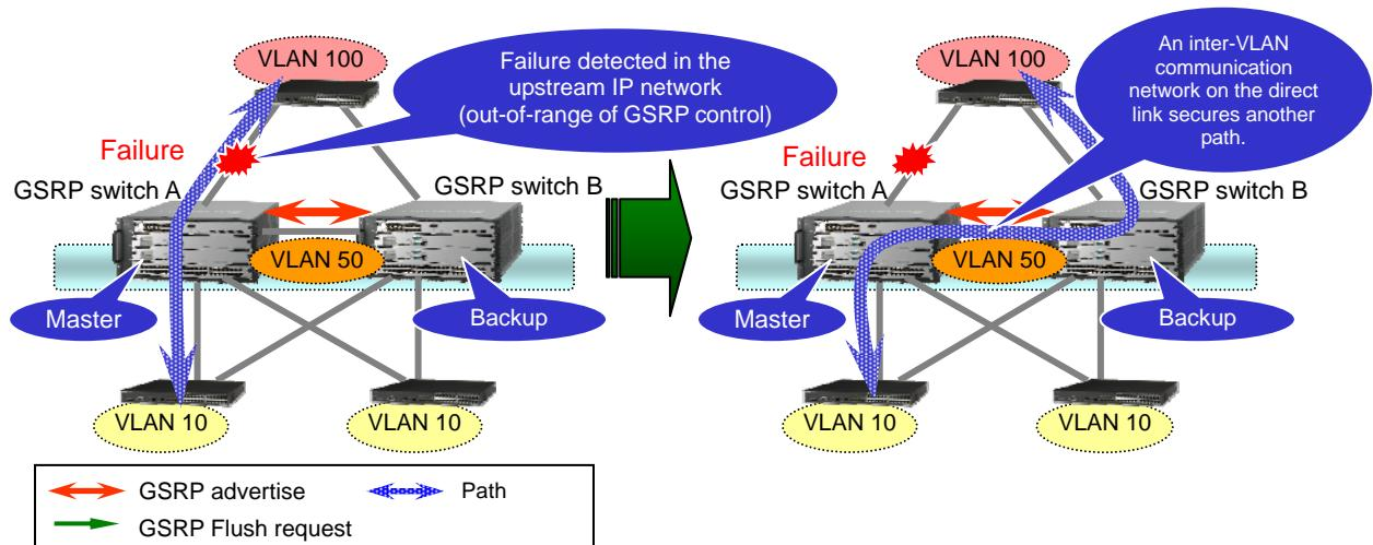
**Figure 1.2-3 Operations in case of a line failure with an upstream IP network**
