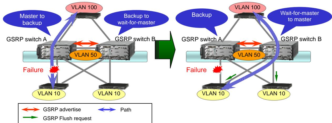
Figure 1.2-1 Operations at the time of link failure
