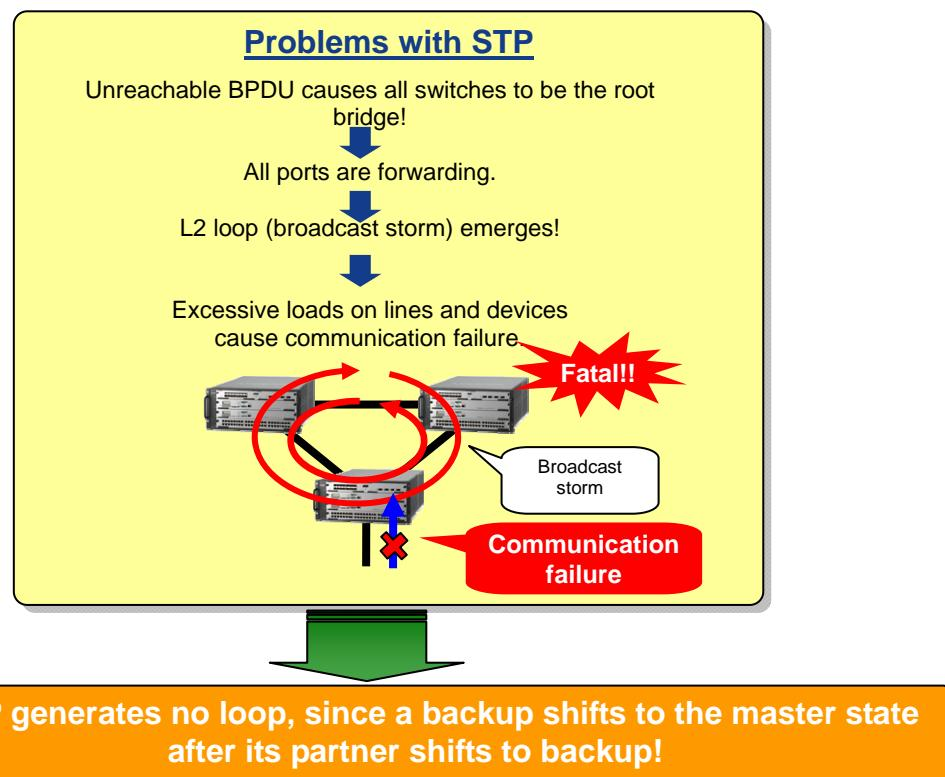
Figure 2.1-1 The problem of overlapping masters in STP
