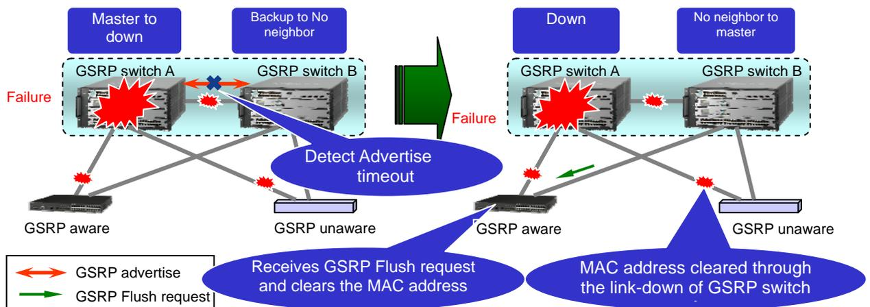
Figure 1.2-2 Operations at the time of master device failure
