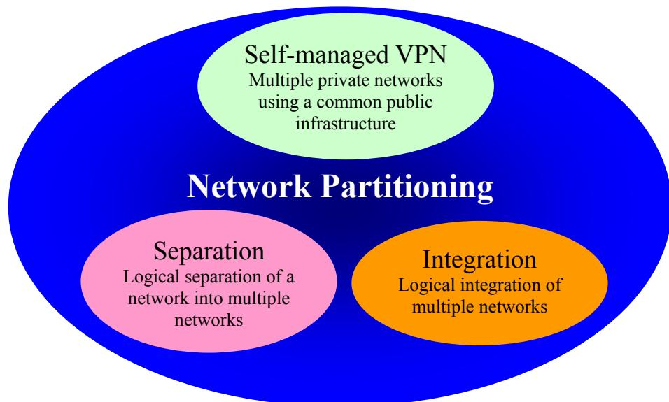
**Figure 1.1-1 Three scenarios where a network partition is recommended**
