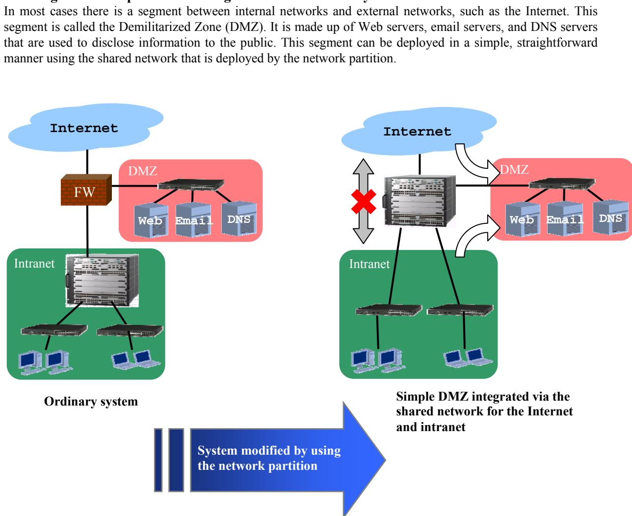
**Figure 6.2-1 Using the network partition to integrate a DMZ into the system**
