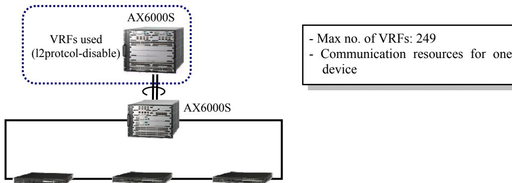
**Figure 6.1-2 Ring separated from the system**
