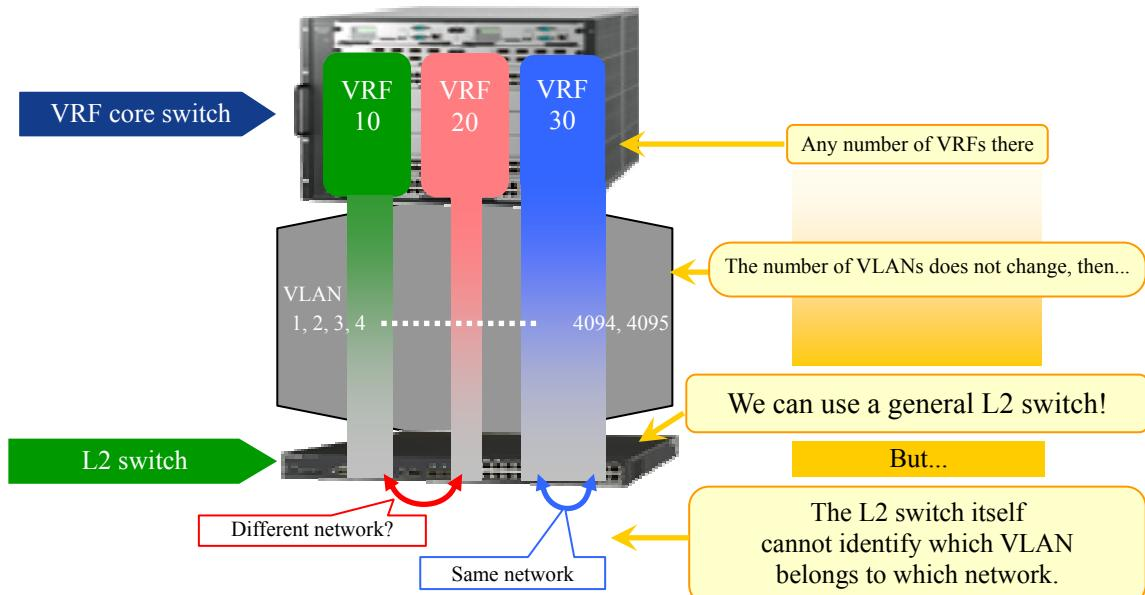
**Figure 2.1-1 VLANs in a network partition**
