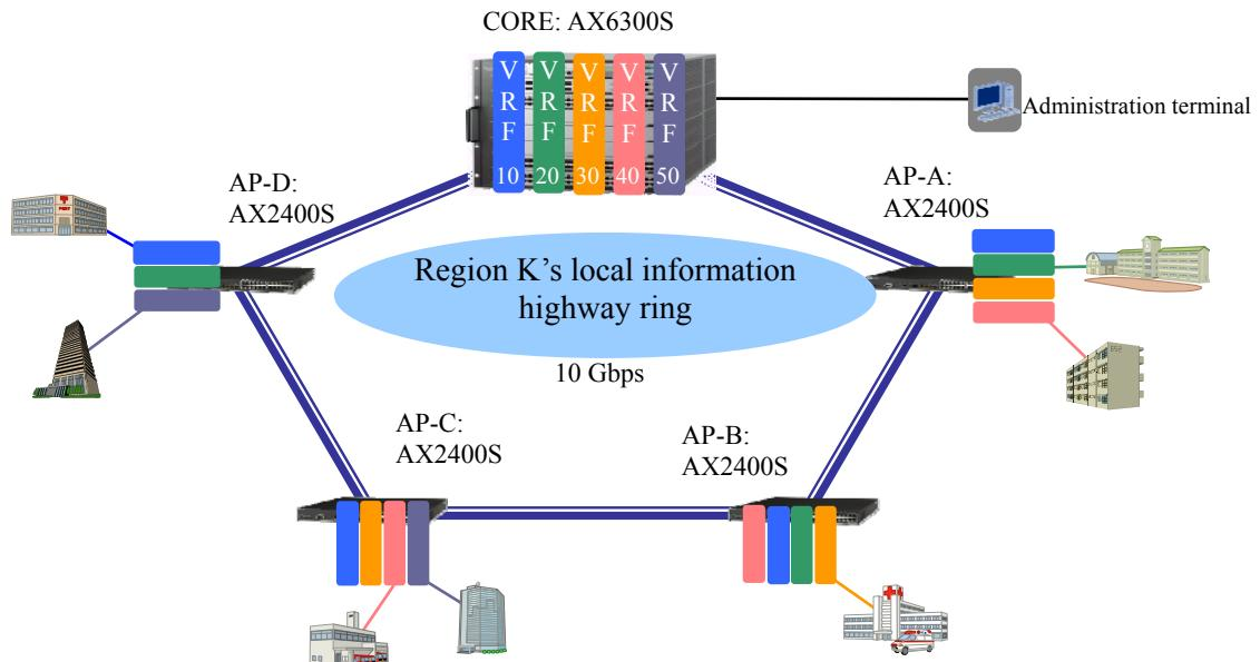
**Figure 3.3-1 Self-managed VPN using network partitions and a ring network**
