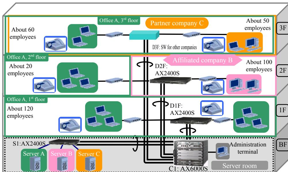
**Figure 5.3-1 System integrating the company networks**
