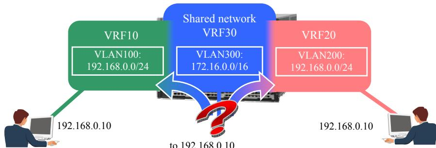
**Figure 2.2-2 IP addresses cannot be identical when using a shared network**
