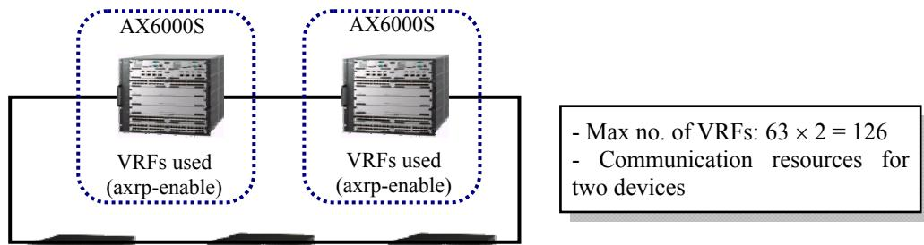
**Figure 6.1-1 System with two VRF devices installed**
