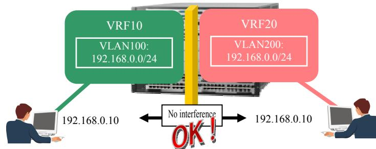
**Figure 2.2-1 IP addresses can be identical**
