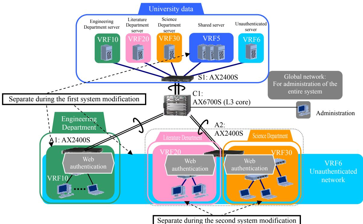
**Figure 4.3-1 Separating the departments with network partitions**
