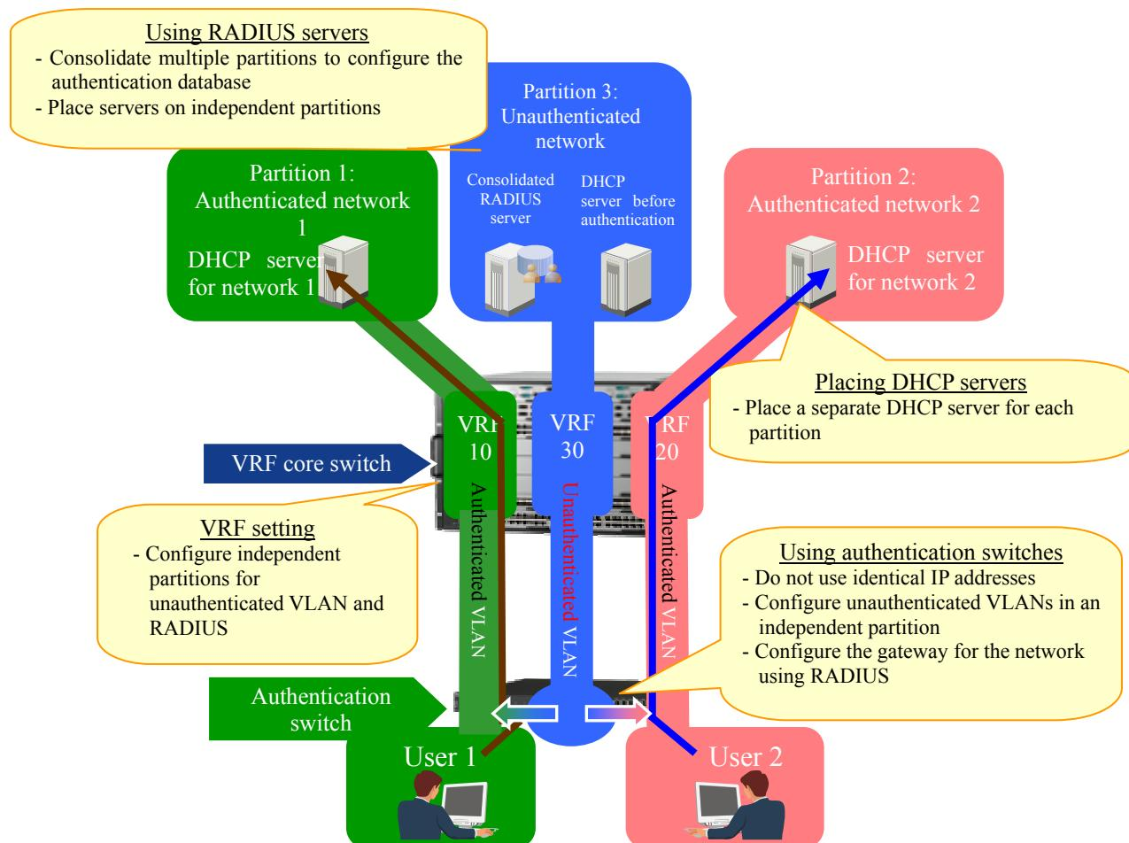
**Figure 2.3-1 Recommended configuration for handling multiple networks with a single authentication switch**
