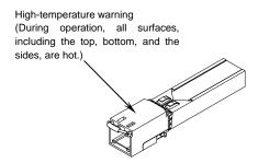
To remove the SFP-T transceiver, use the procedure below. Failure to do so could result in burns.
