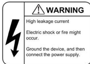
If you use a DC power supply, always connect the ground terminals. Using the Switch without grounding could result in electric shock or failures due to electrical noise.
