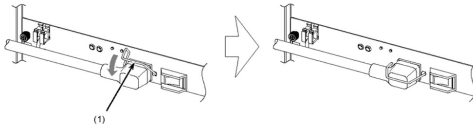
(1) Bracket preventing disconnection of the power cable
