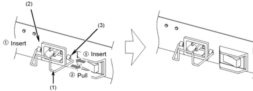
(1) Bracket preventing disconnection of the power cable
