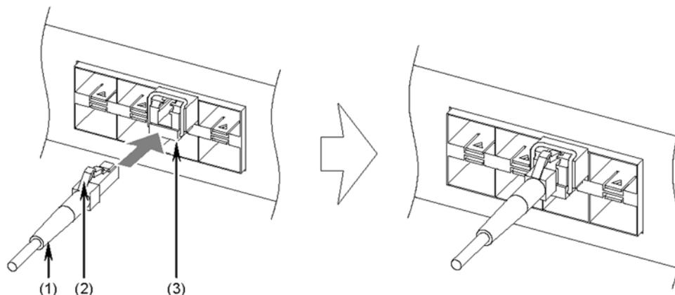
(1) Fiber optic cable (LC simplex connector)
